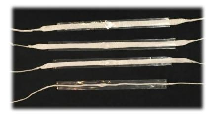
The best is to select the most resistant ligament compatible with the size of the bones and tunnels which can be made, and the inter-condylar notch must be wide enough to avoid any risk of friction.
