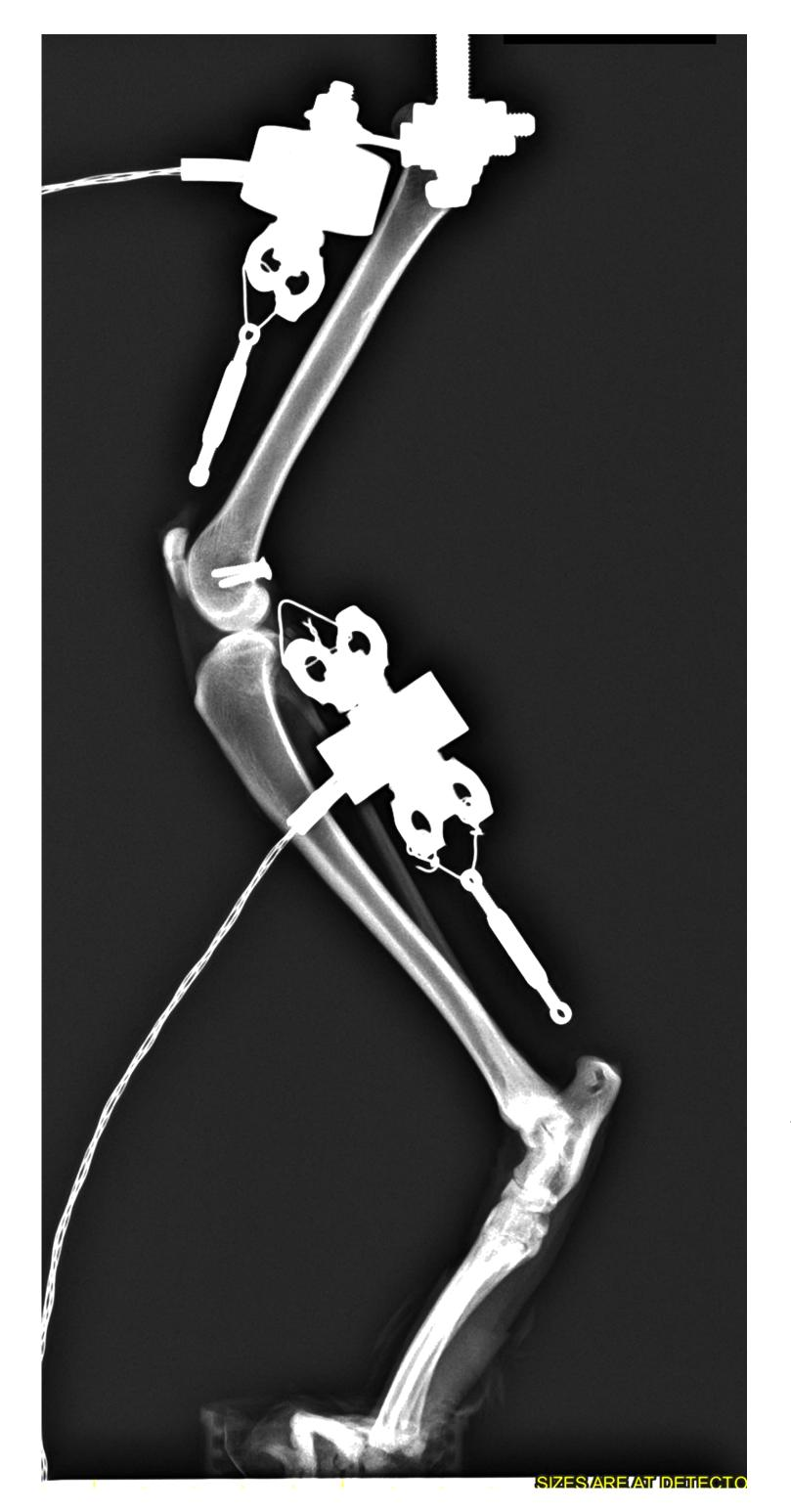
LEFT: Example of limb mounted in limb press. The proximal attachment allows flexion-extension movement but constrains rotation. Load cells are visible connected to an Arduino Uno.
